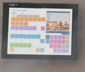
K5 has been tested and certified to be dust-tight and protected against powerful jets of water. A Kitchen Display System (KDS) with an IP66 rating is designed to withstand harsh environmental conditions. It provides real-time information and data to enhance kitchen efficiency.
